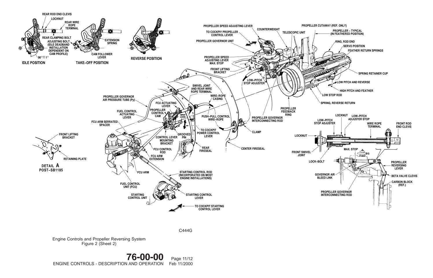
However, on selection of reverse power the lever pin moves into the radial section of the cam slot, rotating the propeller control cam and transmitting this motion forward through the push-pull wire rope to the propeller reversing lever.
